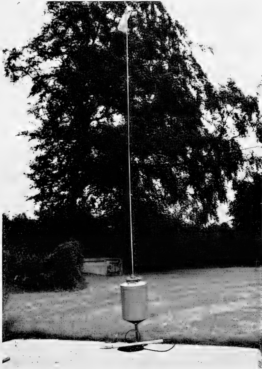
Fig. 4. A photograph of a sono-radio buoy and hydrophone. The 8-ft-long bottom pole, made from galvanized iron tubing, is not shown.
